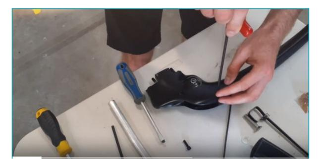
1.3 Clamp the assembly by the Front Tiller Arm in a vice using soft jaws
