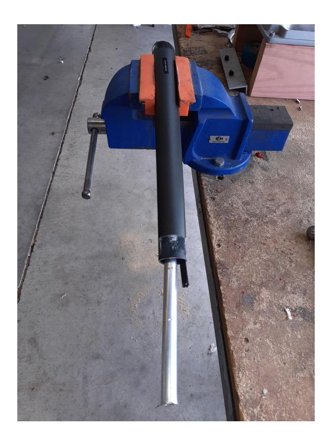
1.5 Front Tiller Arm separated from Tiller Junction for rebuild.
