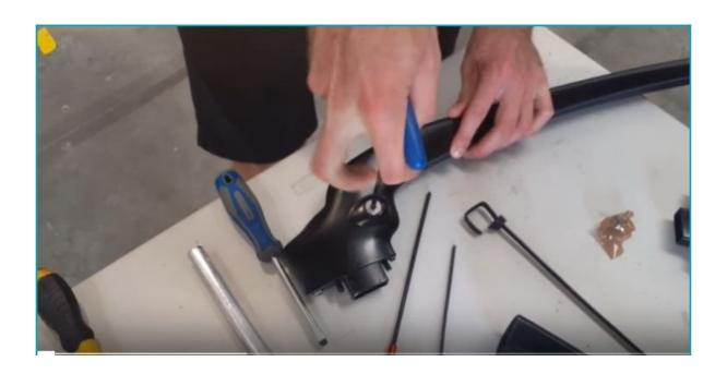
1.3 Remove M5 screws that hold Pivot Junction LH and RH sides together
