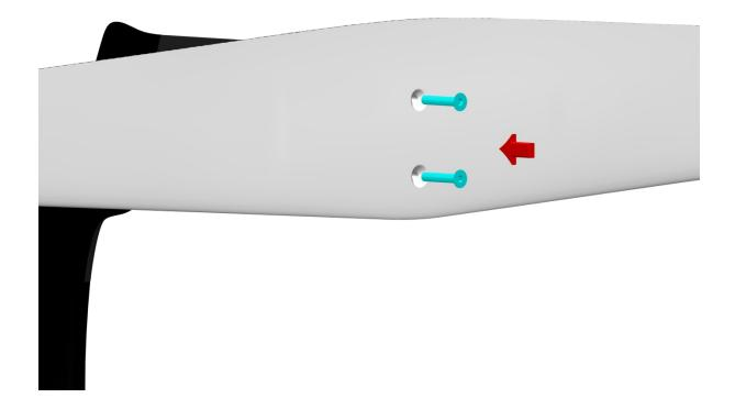
2.4 Fasten the two M6 countersunk stainless steel screws by rotating clockwise. [Tools: 4 mm Hex]
