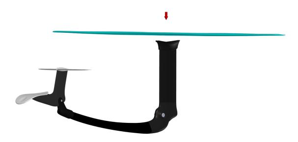
2.3 While holding the Front Tiller Assembly and Front Foil in position, insert the new 35mm length countersunk stainless steel replacement screws into the holes aligning with the Front Foil Shoe and threads on the Front Tiller Strut (aluminium extrusion).
