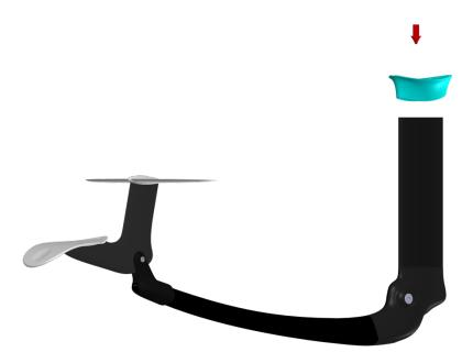
2.2 Position the Front Foil with leading edge (rounded edge) facing forward and holes aligning with that of the Front Foil
