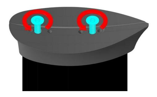
1.2 Remove the Front Foil Shoe from the Front Tiller Assembly and clean off any sand that may have collected between the Front Foil Shoe and Front Tiller Strut (aluminium extrusion).
