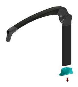
**INFORMATION:** Sand and grit working its way in between the Front Foil Shoe and Front Tiller Strut can make it harder to remove the shoe. Tapping the aft end of the shoe with a Rubber Mallet or using a plastic or wooden block is an effective method for removal.
