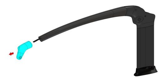
**INFORMATION:** Inspect the Mini Tiller Pivot for damage. Too much play in the fitting to the Front Tiller Arm is not desirable and can be corrected by replacing the Mini Tiller Pivot.
