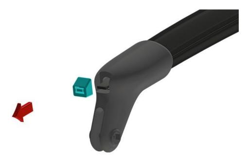
**INFORMATION:** The zip tie parts are not intended to be re-usable and has to be replaced after removal of the zip tie head/late
