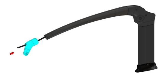
**INFORMATION:** It is acceptable to apply a layer of black PVC electrical tape to the end of the Front Tiller Arm to improve the tolerance and fit between Front Tiller Arm and Mini Tiller Pivot.
